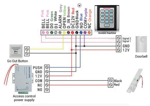
Note: The power controller needs to be connected to 220V, other accessories can be connected with network cable
